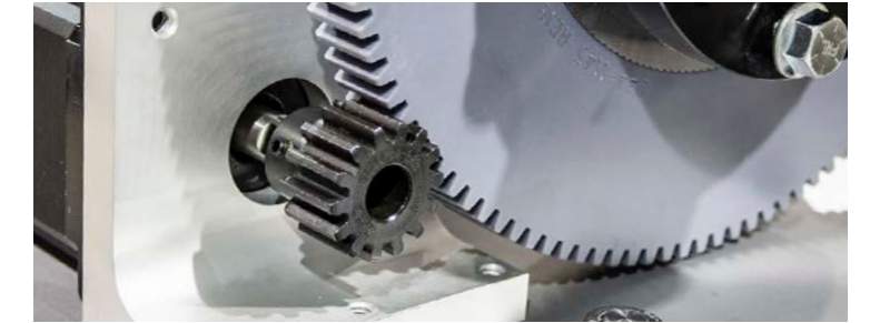
Y-Axis: A gear driven system that rotates the material.
