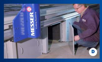
Table doors allow for easy lost part retrieval and slag removal.
