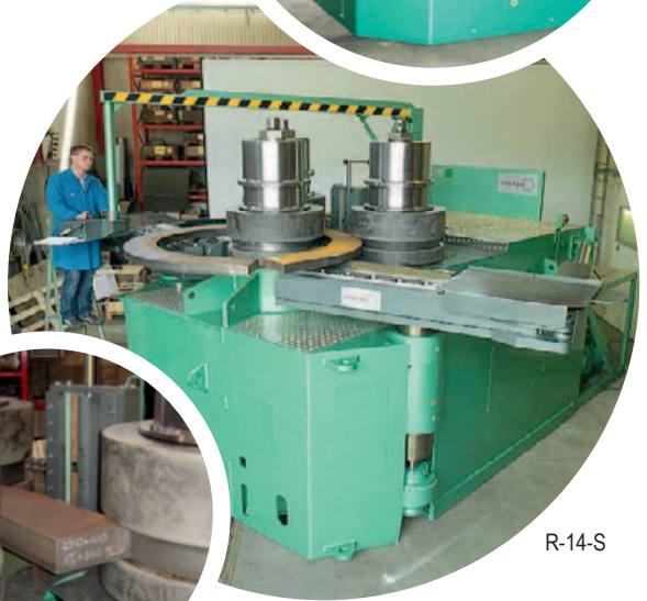
R-14-S Bending flat bar 250x100 mm (10" x 4")
