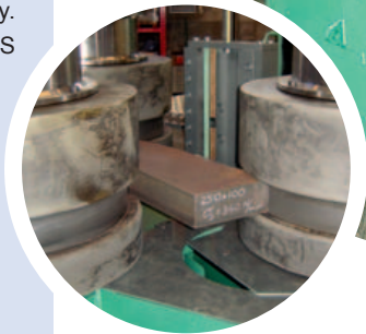
R-14-S Bending flat bar 250x100 mm (10" x 4")
