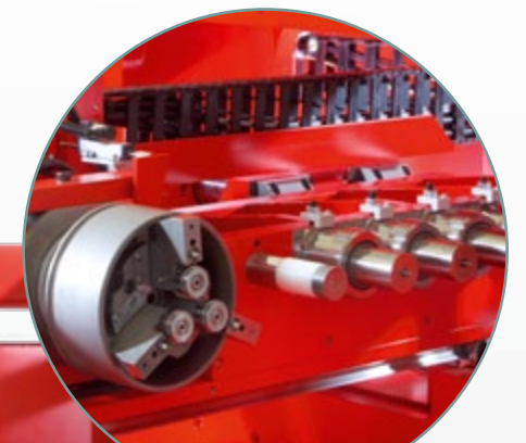
Tool magazine with forming tools and rotary forming unit
